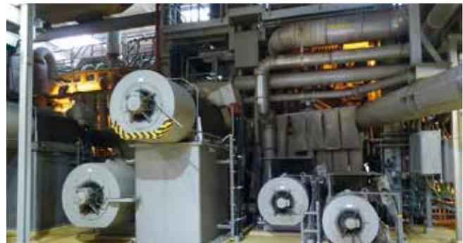
Paper machine with *WebDrive®/Paper* sectional drive from the drive side
