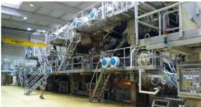
Paper machine with *WebDrive®/Paper* sectional drive from the operator's side
